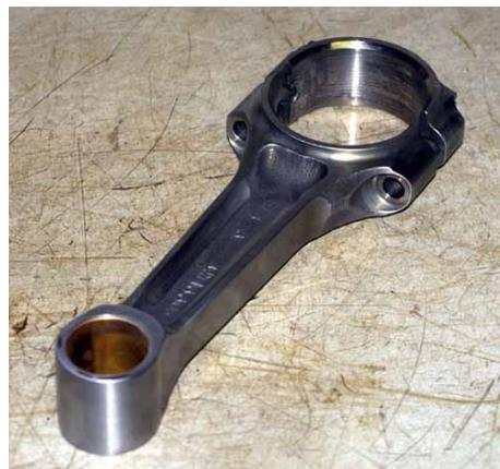
The conrods were fine - nothing to wear on them as the bearings are separate - and were re-used after non-destructive testing using a magnetic field method to check for cracks. The conrod bolts were replaced with new, this is mandatory.
