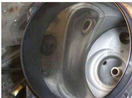
Some cylinders were a lot better, with the corrosion only just visible. Fortunately, the corrosion was not as bad as it looked. It was smooth to touch and not deep enough to require a rebore; it came out with a standard re-hone which should always be done anyway whenever piston rings are changed.
