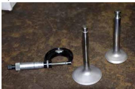
The exhaust valves were about 0.002" undersize on the stems - this is within overhaul limits but outside new limits - and were replaced; a significant item at \$200 each. The exhaust valve stem is filled with
