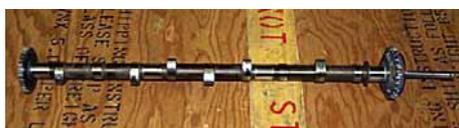
It was reground to new factory limits as Barrett Precision rebuild an engine to these not to overhaul limits which are looser. This is a bonus over what one normally gets in an overhaul from elsewhere but it does mean some parts are discarded when they could have been re-used in a legally overhauled engine.
