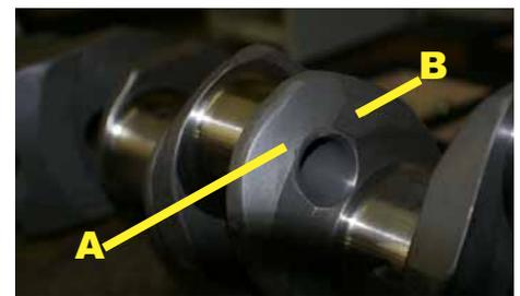
The illustration above shows some of the areas (A, B) where Lycoming remove metal (a lot of it; 5-10mm in thickness) to dynamically balance it, to 15 gram-inches. The illustration below shows additional surprisingly rough machining by Lycoming.
