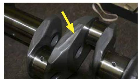
The original crankshaft is nitrided - this is a surface hardening process which yields a hard-wearing surface while preserving a tough core. The additional machining done by Barrett Precision is done in similar areas to A/B; less than 0.010" of metal is removed and if more needs to be removed the crankshaft is re-nitrided.
