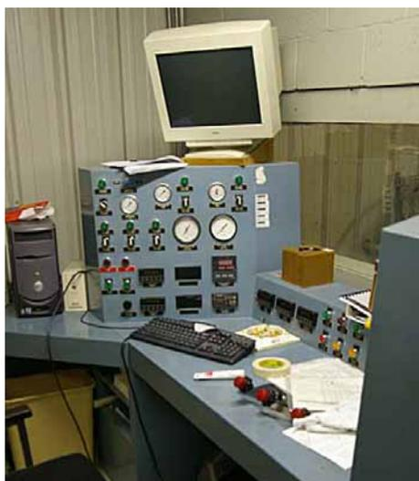
The dyno run turned up a problem with the fuel servo: the fuel control valve was not closing properly, causing a shudder at shutdown. This surprised me, as the shudder had always been present, and is usual with these engines. However, according to Barrett, this is not how it should be.
