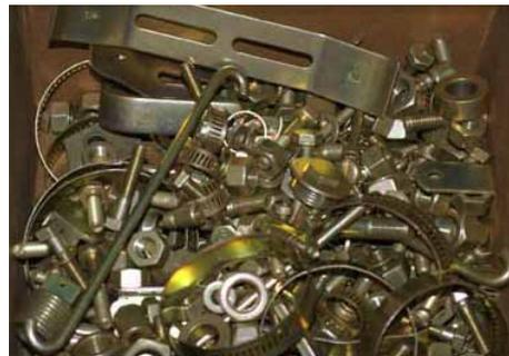
Most engine shops, Lycoming included, assemble the engine and spray over the whole thing, covering all the bolts and other fittings. Barrett paint the major engine parts (cylinders, crankcases) separately and install the fittings (screws etc) afterwards. The original fittings were largely re-used after replating as shown in the photo above and this results in a much cleaner looking engine.
