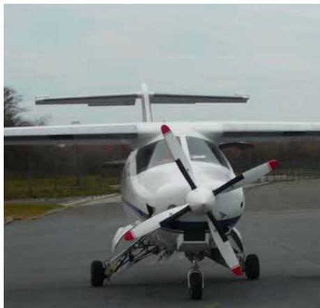
*The extra 400. Similar to the 500 but with a 350hp piston engine and four-blade prop*
