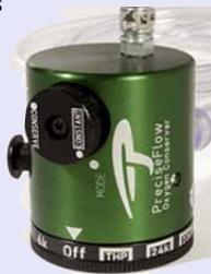
Tested at the standard FL180 setting, it achieved the best oxygenation of all systems (90-94%). Oxygen usage was 80 l/h, a 47% saving. When reviewing the test results later, we also discovered that the pressure regulator used has a slightly higher pressure than recommended by PreciseFlow. Compensating for that, a saving of ~55% would be realistic while still giving 90% saturation.
