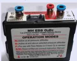
system has a built-in pressure sensor. Instead of setting the system to an altitude, you just switch it on and set the altitude at which you want the flow to start – always on, 5,000 or 10,000ft. This has the added advantage that you don't waste oxygen during climb. On the other hand, it needs electrical power (3 AA batteries or an optional external power supply), and if that or a part in the "magic box" fails you are stuck with no oxygen, as the system fails "off".
