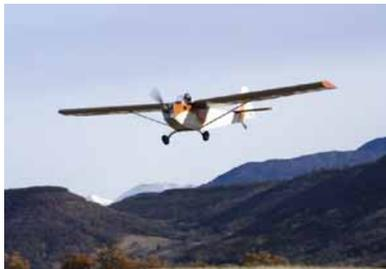
During the flight the aeroplane travelled 50 km. This is a major achievement in the search for environmentally friendly aeroplanes and travel. Hitherto several aircraft powered by batteries have flown. However, Electra is the first aeroplane with batteries that will qualify for an airworthiness certificate and the first aeroplane to fly for 48 minutes without any additional sources of power, solar or otherwise.
