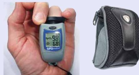
*Pulse oximeter showing 98% oxygenation and heart rate of 68, with carrying pouch*
