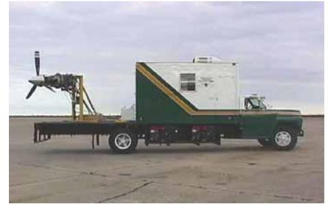
*The test rig used in the Baylor University study, complete with PT6A-6 turbine engine*
