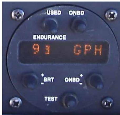
Picture 1. Shadin fuel computer from a TB20
