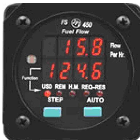
Picture 3. Dedicated fuel flow readings can also be provided with the JPI 450
