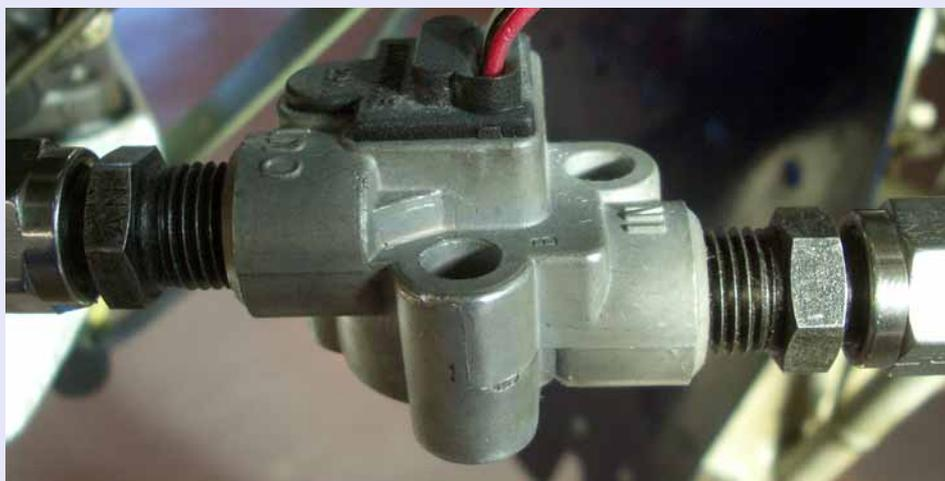
*Typical fuel flow transducer used in light aircraft*
