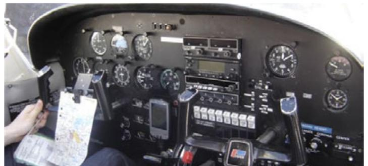
*The combined com and ADS-B radio is the second from the top*
