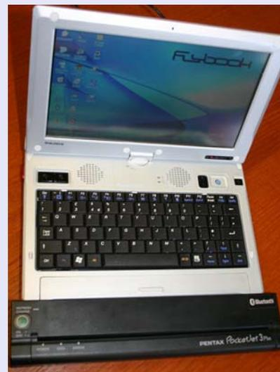
*The Pentax Pocketjet provides one of the smallest printing solutions available measuring just 2" by 1" cross section and 7" long*
