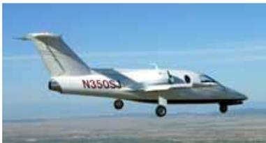
Performance goals include 340 knots at 25,000 and a 900 nm range. Unfortunately, the company suffered a setback when the prototype crashed on takeoff for its 25th test flight. Both pilots were unharmed.
