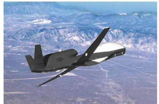
Unlike the U2, it is unmanned and can stay aloft for more than 32 hours at a stretch. It is launched with a single mouse click and the plane carries out the entire flight autonomously. A recent innovation by Northrop Grumman, makers of the Global Hawk, puts a file server and military radio on board. This allows front line grunts to call up images from the plane in real time using a PDA connected to a radio modem. "It's just like MapQuest," says the manufacturer.
