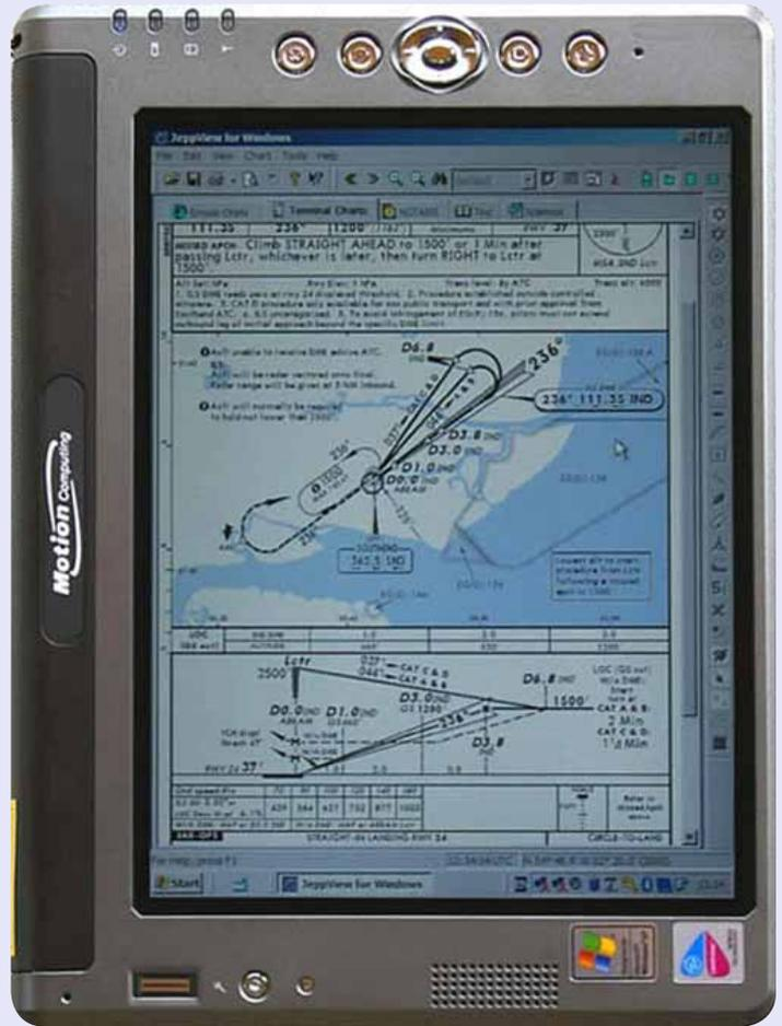
For night operations, a very low brightness level is essential and most portables fail in this miserably. The LS800 does this acceptably but you need the manual brightness control to get it low enough. Some GPS moving map applications (not Jeppview as far as I can tell) offer a "night vision" mode where the primary display colour changes from white to red.
