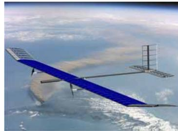
The Mercator, an un-crewed plane with a 16m wingspan, will cruise the stratosphere for weeks or months at a stately 20-30 knots. Made out of carbon fibre, it is powered by solar cells. During the day they drive the two propellers and charge batteries for night operations. A 40 percent
