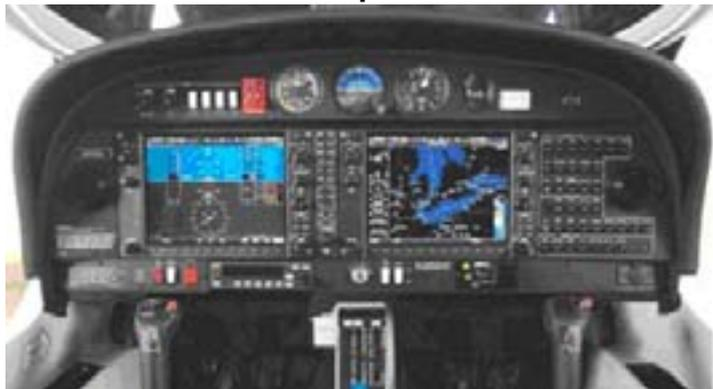
Diamond's DA40 is the platform for the first certified Garmin G1000 glass cockpit installation. With everything you'd normally expect on a PFD and multifunction display, the G1000 also features digital audio, a WAAS-capable IFR GPS, VHF navigation with ILS and VHF communication with 8.33KHz spacing. The whole package is run from a solid-state attitude and heading sensor, and can have Mode S, weather and terrain data display added on.
