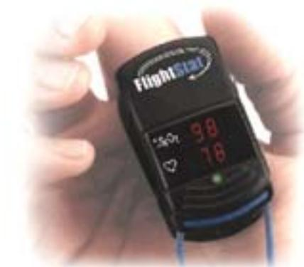
**The FlightStat Pulse Oximeter** emits red and infrared light through your finger and detects the fluctuating signals caused by the pulsating blood flow. Your pulse rate is determined from the signals received by a light detector. The ratio of the fluctuation of the red and infrared light signals is used to calculate your blood oxygen saturation (%SpO<sub>2</sub>) of hemoglobin
