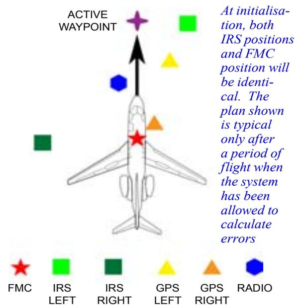
*At initialisation, both IRS positions and FMC position will be identical. The plan shown is typical only after a period of flight when the system has been allowed to calculate errors*
