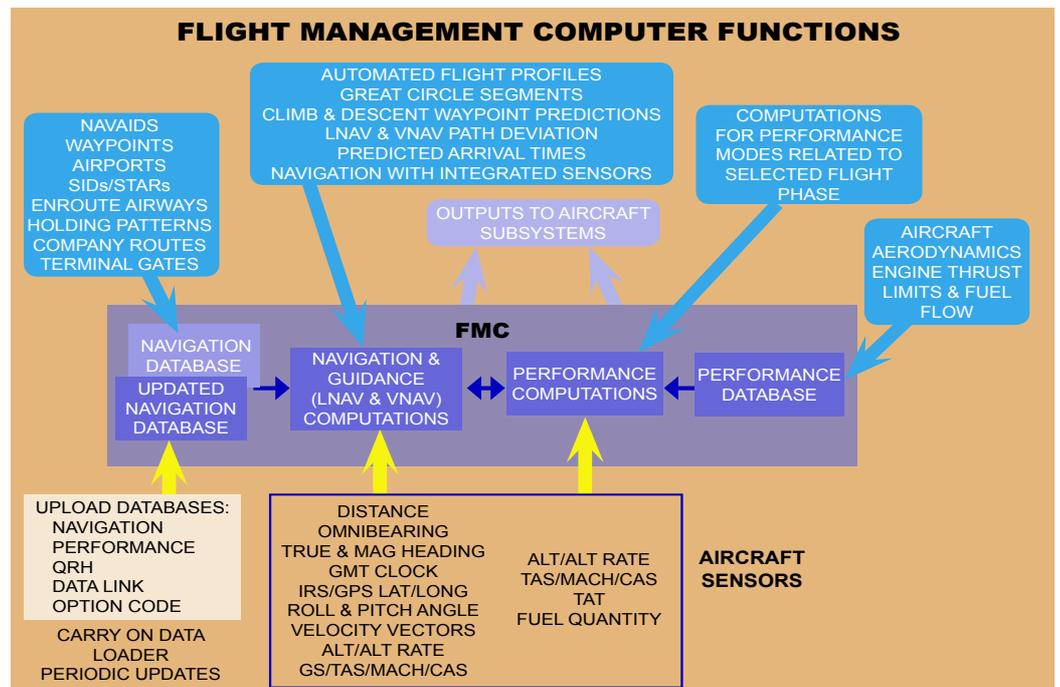
erroneous estimates from the raw input data i.e. the FMC rejects bad data from an individual sensor if that data does not compare favorably with the others.
