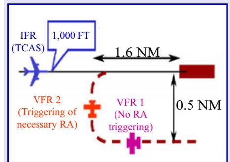
In the example shown in the diagram above, provided that the lateral distance between the final approach path and the downwind leg is at least 0.5 NM, the VFR traffic on the downwind leg (VFR 1) will not trigger an RA on board the TCAS-equipped IFR traffic on the final approach. (In addition, TCAS does not generate any RA below 1000 ft.) If the IFR on the final approach receives an RA, this confirms that the separation with the VFR traffic on the base leg (VFR 2) is inadequate.
