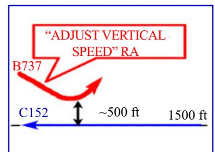
In Class A airspace, a B737 is descending on the glide path for the final approach.
