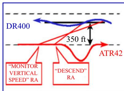
Subsequently, the RA is strengthened into a “Descend” RA when the vertical separation between the aircraft becomes less than 350 ft. The pilot follows the RA and descends to FL57 before climbing back to FL60.
