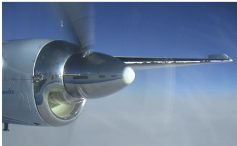
*Two degrees of ice: The effect of climbing through light to moderate mixed ice in February. De-icing on leading edges and anti-icing on air intakes are working well, but ice has built up on the tips of spinners*
