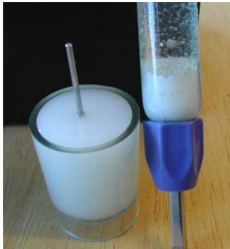
*This milky looking substance is caused from mixing water and diesel*
